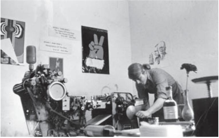
Figure 13: Chip Berlet using the College Press Service ATF Chief 15 offset printing press in Denver, Colorado. (c) 2012 Chip Berlet
